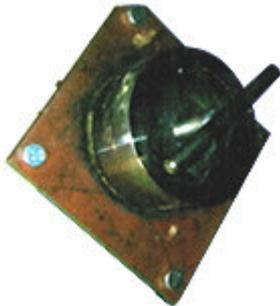
Simple, secure coupling devices are mounted on the equipment in areas of known build up, which allows you to set the Cardox Tube to a predetermined depth and discharge direction.
