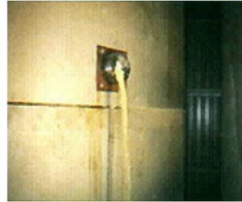
After: The tube is removed to reveal build-up has been cleared and product is aerated and once again free flowing.
